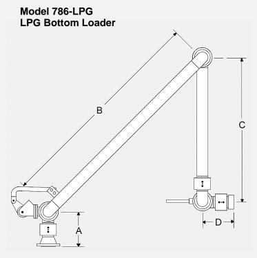
The Model 786-LPG is produced specifically for LPG service. A solid construction design with full penetration welds, the components are made with uniform ASTM schedule 40 specifications, a 300# ANSI inlet flange connection and a 3000 lb. heavy duty outlet coupling.
