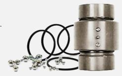
Designed as the basic workhorse of the swivel joint world, the 80 Series is a ball bearing, single point seal design with a felt dust seal backup that allows for an endless number of applications. The 80 Series is available in carbon steel, stainless steel T-316, and aluminum. Sizes range from 2" to 6" in all materials. In addition, an 880 Series cast aluminum variant is available which can help reduce overall cost yet maintain the overall o-ring series characteristics.
