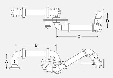
The Model 752-F is a low profile fueling transfer design. Adjustable for varying elevations and degrees of loading, the standard riser swivel point is at ground level with optional custom supported positions. The torsion spring mounting bracket is nestled within the assembly silhouette for tight spaces. Secondary arms can be installed in either an upfeed or downfeed position, as required by customer specifications.
