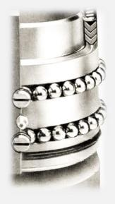
The unquestionable sales and performance leader of the OILCO swivel joint line. The 90 Series swivel joint is designed with a three "V" ring seal configuration that is spring loaded and self-adjusting for normal wear. The incorporation of these "V" rings maintains a constant optimal pressure, securing a reliable seal long after conventional single rings or compression seals may be compromised.
