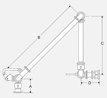
The Model 754-FR is the rigid version of the flexible hose bottom loader. This A-Frame loader conforms to the recommended API envelope for modern truck construction. The Model 754-FR can either be stored in a limited space with reduced dimensions or multiple units can be arranged in a crossover arrangement for up to 5 service positions.
