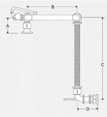
The Model 704-F is the torsion spring counterbalance replacement for traditional slide weight style overhead loading assemblies. Engineered for short range and compact placement, the 704-F can be offered in a stackable arrangement with varying hose length. For single spaced placement the horizontal length may be adjusted to give maximum articulation range.
