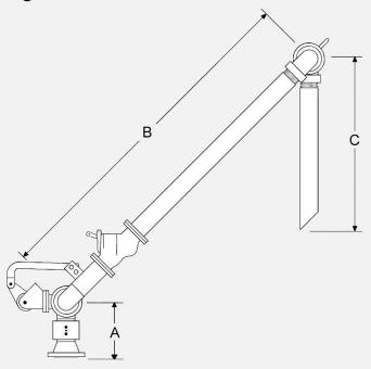
The Model 755-F is the simple and popular fixed reach option for top loading facilities. Standard torsion spring counterbalances offer extended service life, minimal adjustments over time, and a limited swing radius necessary for multiple positions. An optional remote control handle is available for single operator spot filling procedures.
