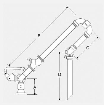
A replacement option for the antiquated sliding sleeve style top loader, the Model 756-F Pantograph is a dry line assembly designed to operate over varying manhole locations. reaches. Extension ability up to 9'6" for standard arms, while extended reaches can be afforded in the 1156-F model. Standard materials of construction are carbon steel and aluminum with an optional remote control handle for the horizontal deadman valve.
